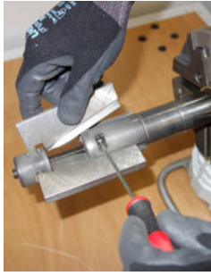
Quick setting of the pipe dimension
