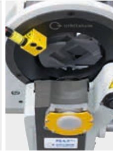
Additional saw blade position for cutting off tube elbows
