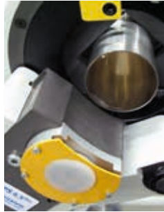
Tried-and-tested planetary cutting principle: The saw blade immerses into the cut and is guided orbitally around the pipe
