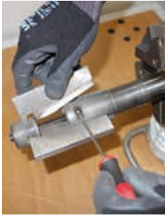
Quick setting of the pipe dimension
