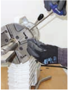
Quick tool change clamping system OTC®
