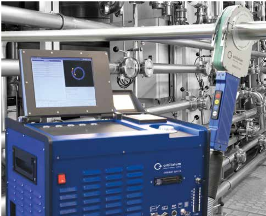
10.5" swivel monitor and system printer integrated
