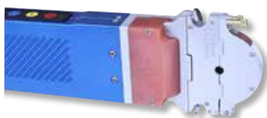
ORBIWELD 12 with narrow clamping cassette (Type "A")
